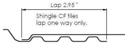
Figure 12.4 Side Lap Detail
